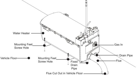
Fig. 27 Place the Water Heater On The Floor
