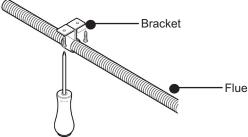
Fig. 18 Attaching Flue Bracket
