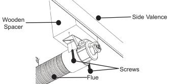
Fig. 16 Attaching the Flue Terminal to the Vehicle
