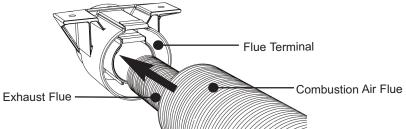
Fig. 15A Attaching Flue To Flue Terminal
