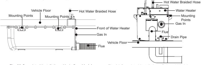
Fig. 33 Completed Installation - Underfloor Models
