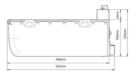
Fig. 4 Dimensions – Side View Underfloor
