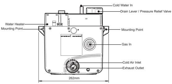
Fig. 2 Dimensions - Front View Underfloor
