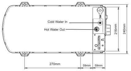
Fig. 3 Dimensions – Plan View Underfloor
