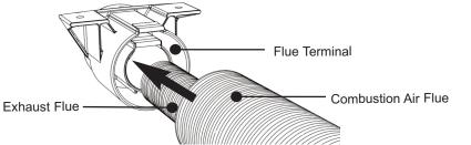
Fig. 23A Attaching Flue to Flue Terminal
