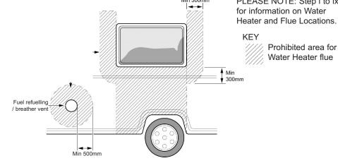
Fig. 8 Installation Locating Diagram - Underfloor Installation
