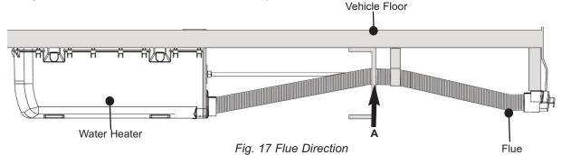
The flue **must be** attached to the underside of the vehicle floor with the two brackets supplied. Clip the bracket around the flue and use two screws (No.8 x  $\frac{3}{4}$ ") to secure each bracket to the underside of the vehicle floor as per Fig.18.
