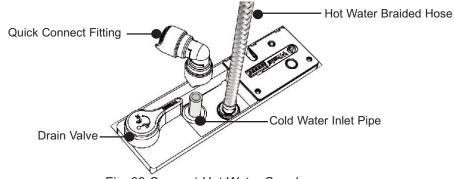
Fig. 32 Connect Hot Water Supply
