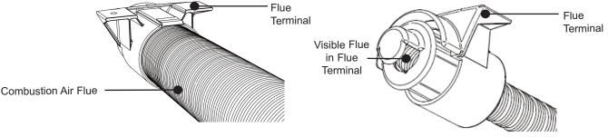
Fig. 23B Attaching Flue to Flue Terminal
