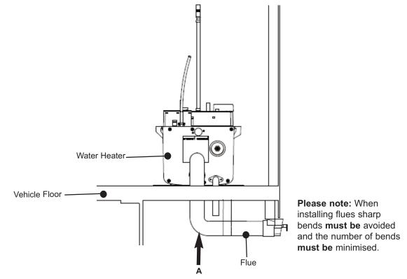
Fig. 25 Flue Direction
