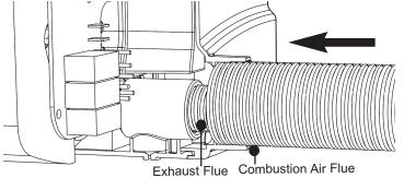
Fig. 22 Attach Combustion Air Flue
