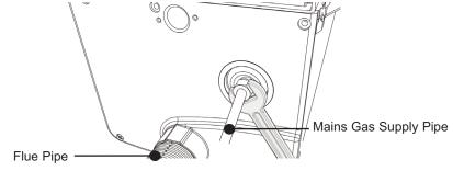
Fig. 29 Connecting Gas Supply
