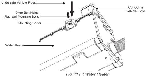
iii. Secure the mounting bolts with M8 serrated flange head nuts (not supplied).
