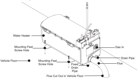
Fig. 28 Secure the Water Heater To The Floor
