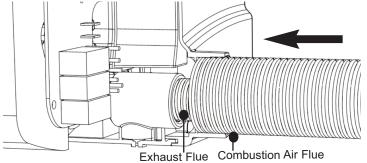
Fig. 14 Attach Combustion Air Flue
