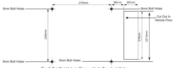
Fig. 9 Cut Out Hole in Floor - Underfloor Installation
