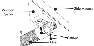
Fig. 24 Attaching the Flue Terminal to the Vehicle
