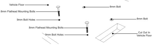
Fig.10 Fit Mounting Bolts
